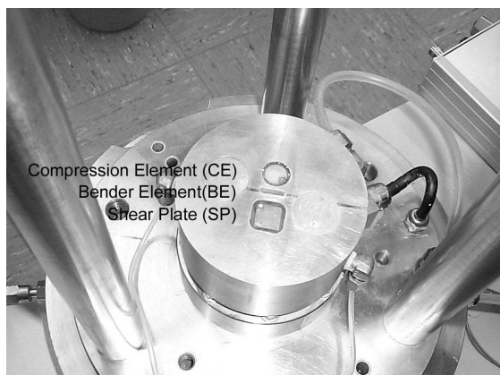
Figure 4.10: Photo of the specimen end plates with piezoelectric elements
