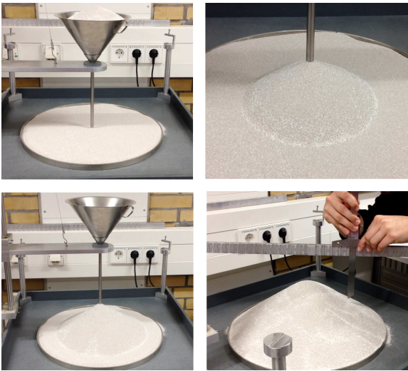
Fig. 8: Determination of the angle of repose \varphi_r from a loosely pluviated cone of sand
