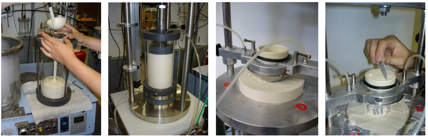
Fig. 2: Preparation of reconstituted triaxial samples of Kaolin via slurry consolidation
