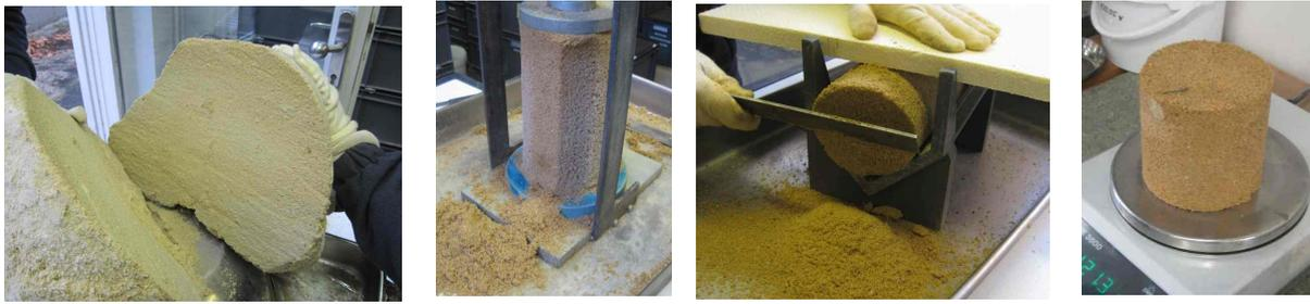
Fig. 10: Preparation of triaxial samples ( $d = h = 100$  mm) out of the frozen blocks
