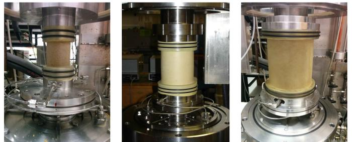
Fig. 37: Samples with different sizes:  $d = h = 50$  mm (left),  $d = h = 100$  mm (middle),  $d = h = 150$  mm (right)
