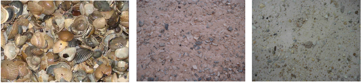
Fig. 1: Photos of a) the shells before crushing, b) mixture SH40 of Karlsruhe fine sand with 40 % crushed shell particles and c) mixture G40 of Karlsruhe fine sand with 40 % coarse sand or gravel particles
